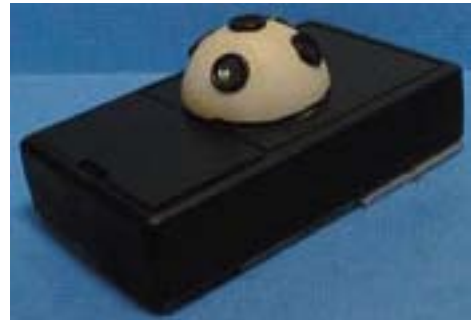
Figura 19 – Transmissor móvel do Active Bat [54]
