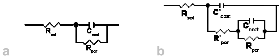
Figure 5.3 Equivalent electric circuits used for numerical fitting of the EIS data obtained for the painted systems: a. undamaged system; and b. two processes.
