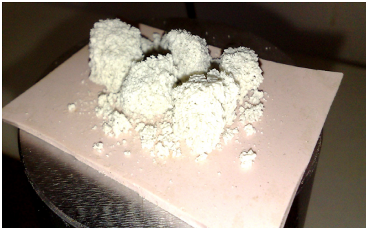
Fig. 4.50: crush of a 30 PPI ceramic foam
