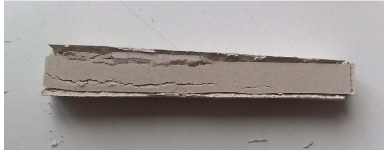
Fig 3.3: dry-pressed bar of 1.7wt.% PVA binder with 15wt.% hydration
