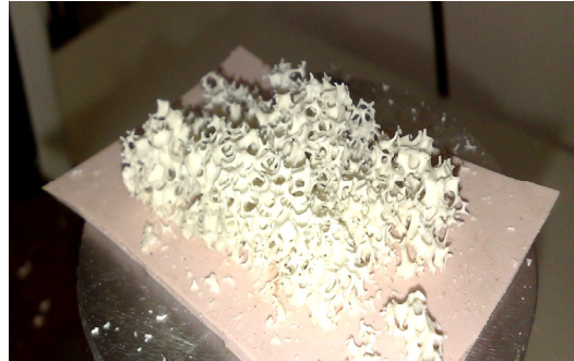
Fig. 4.51: crush of a 8 PPI ceramic foam
