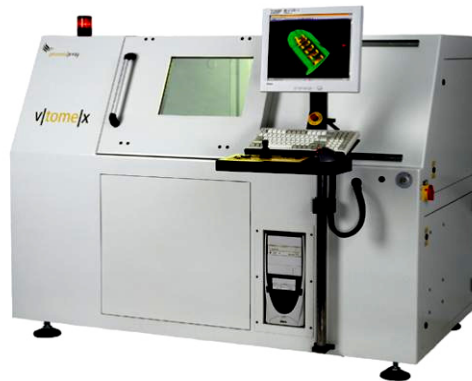
Fig. 4.37: The v|tome|x ultra high-resolution CT system
