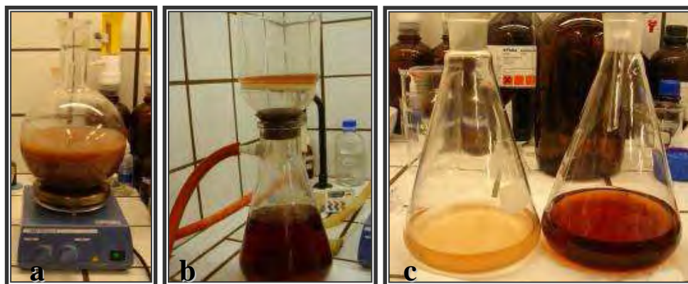
Figure 1.8 – (a) Solid-liquid extraction experiment; (b) filtration with a G3 sintered glass filter; (c) filtrates with a G3 and G1 sintered glass filters.
