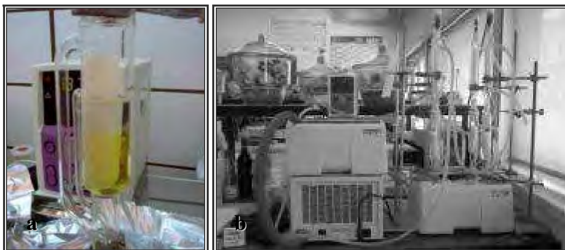
Figure 2.5 – Soxhlet conventional extraction. (a) Soxhlet chamber, first cycles; (b) laboratory scale extraction equipment.
