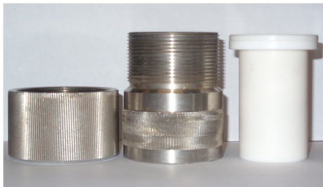
Figure 7.5.: PTFE-lined stainless steel reaction autoclave.
