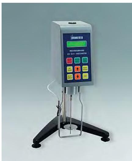
**FIGURA 23 – VISCOSÍMETRO DA BROOKFIELD, RVDV II+ COM 6 AGULHAS**
