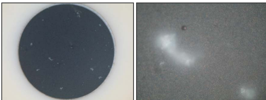
Figure 5.11. Optical micrographs: \times 50 (A.) and \times 100 (B.) of a thin mercury film electrode (7.6 nm of thickness) plated on a glassy carbon electrode, after being used in SSCP experiments with carboxylated latex nanospheres.
