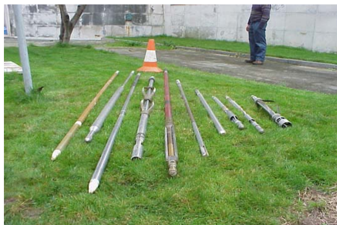
Fig. C.1 Geophysical logging probes used for the depth sampling campaign in the Aveiro Cretaceous aquifer. From left to right: (1) French BRGM Romulus ® magnetic susceptibility/induction resistivity probe; (2) Comprobe ® Inc water sampler; (3) Focused resistivity/gamma ray probe; (4) Heat-pulse flowmeter probe (fitted with centralisers); (5) Caliper, NGAM, SP, point RES probe; (6) MLS single caliper; (7) SIE ® single gamma ray (detector at base); (8 & 9) Sondex ® inline spinner flowmeters (50mm, 30mm) and (10) Geovista ® spinner flowmeter 75mm cage fitted.
