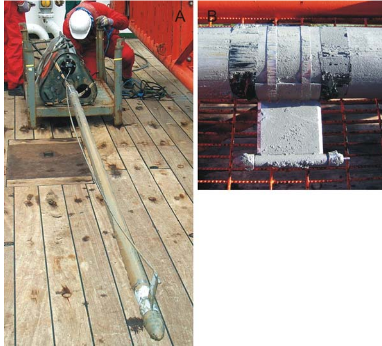
Figure A.4. Heat flow probes. (A) Lister type heat flow probe with a violin bow design used in the GAP cruise and of the same type as the one used during the Anastasya-2001 cruise. (B) mini-temperature logger installed on a gravity corer.
