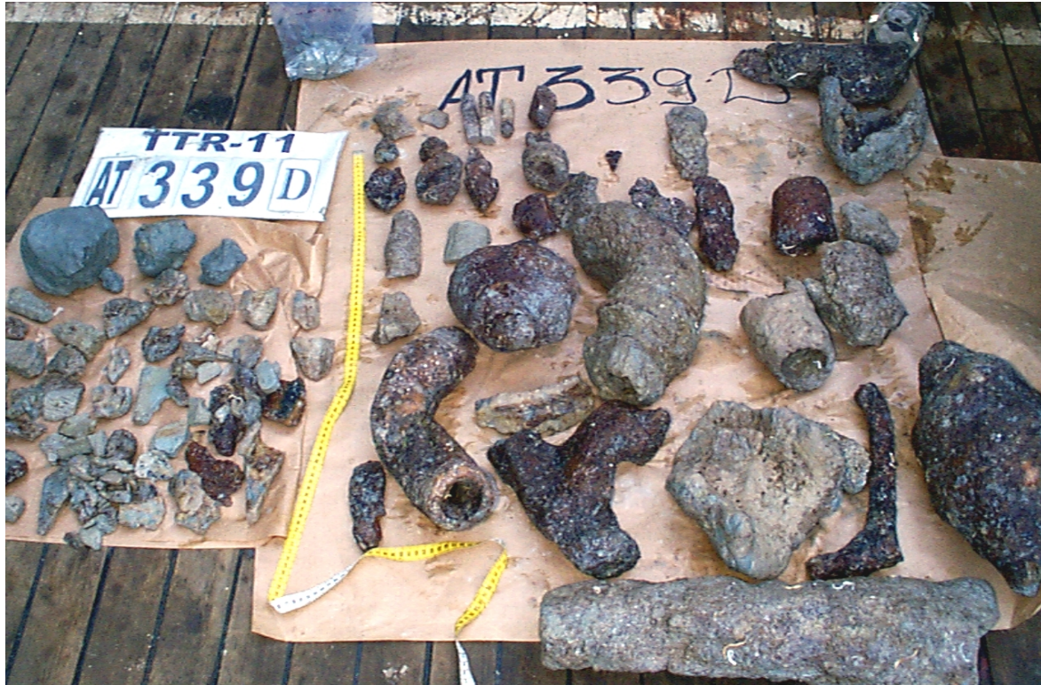
Figure 4.48. Samples collected by the dredge TTR11-339D, with dolomite chimneys and carbonate rubble, composed of fragments of the dolomite chimneys and crusts; also some fragments of claystone interpreted as fragments of the rocky outcrops.
