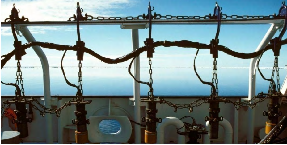
Figure 8 - An array of airguns with different sizes (commons.wikimedia.org).
