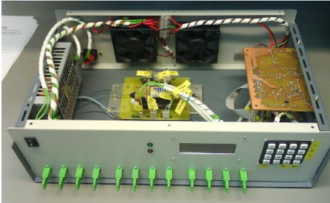
Fig. 3.3 MZI-SOA driving box. The MZI-SOA sits in the middle of the box. The temperature control, SOA bias and phase shifter bias electronics board is on the right, and the power supply unit is on the left. The front plate contains the interface dial, numerical display, and the input (8) and output (4) fibre connectors.
