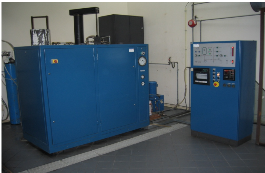
Figure 3-1 – Hot Isostatic Press used for ex situ sample sintering at the Ceramic and Glass Department.
