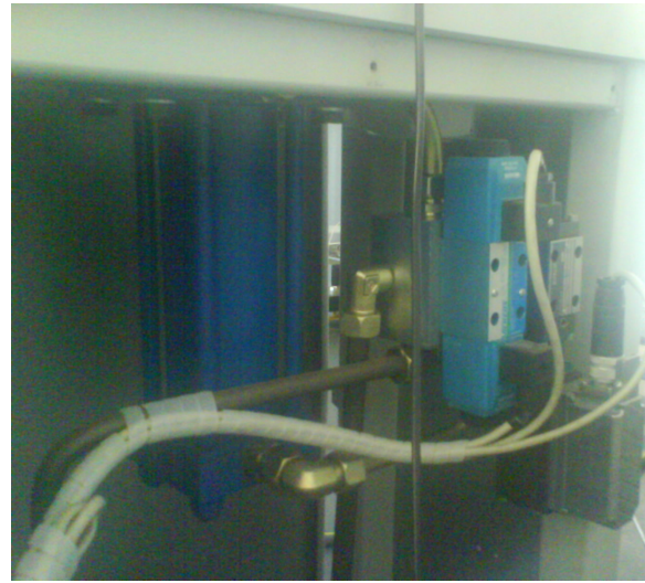
Figure 3: (left) Upper cylinder, valve, load cell and position sensor
