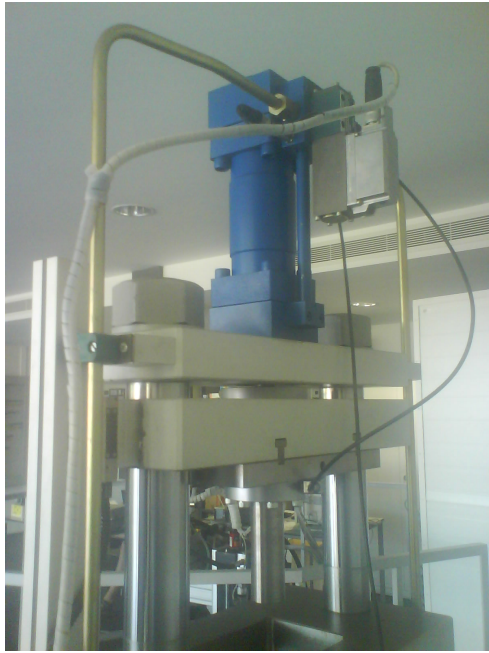
Figure 3: (left) Upper cylinder, valve, load cell and position sensor
