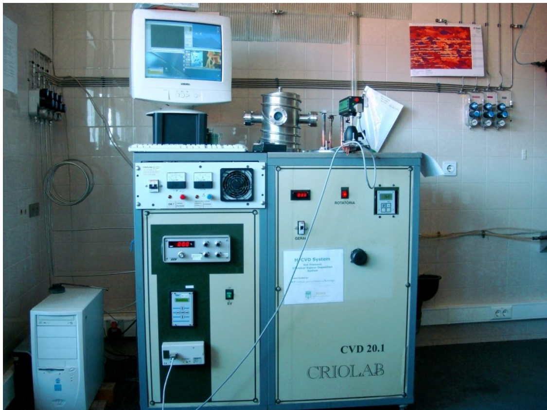
Figure 11 - Hot-filament reactor used
