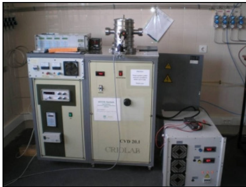
Figure 2.1. HFCVD reactor used for diamond films production [2].
