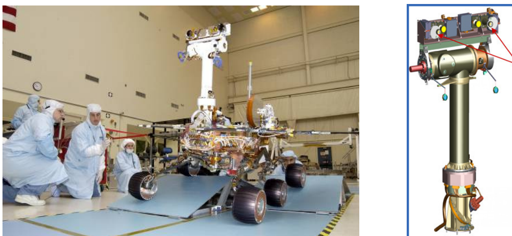
Figure 5. NASA's Mars Exploration Rover (left) also makes use of active perception. The mast (right), where two high resolution cameras are mounted, rotates and tilts. Pictures taken from [MERs homepage].
