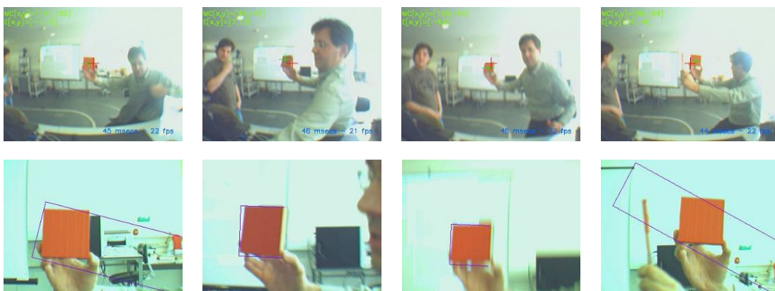
Figure 46. Foveation control by red color recognition. Peripheral view (top row) and corresponding foveal view (bottom row) used to calculate color mask contour.
