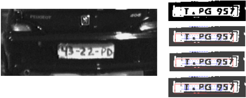
Figure 56. License plate photo extracted from a foveal view Haar detection (left). Debug images for Gnu OCR application (right).
