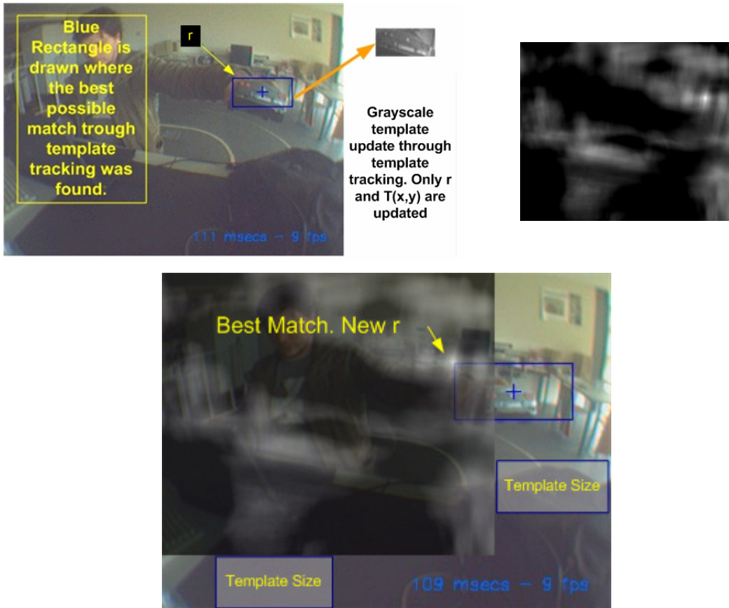
Figure 15. Template tracking (top left) and TMR with the best match in lighter areas (top right). Overlay view (down).
