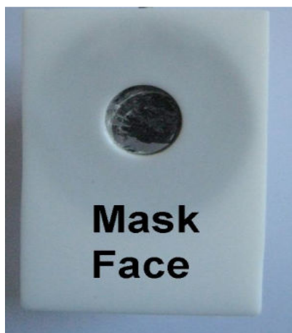
Figure 15: Cell for electrophoretic deposition showing the mask with a 10 mm diameter hole in the centre. [Adapted from reference 40]
