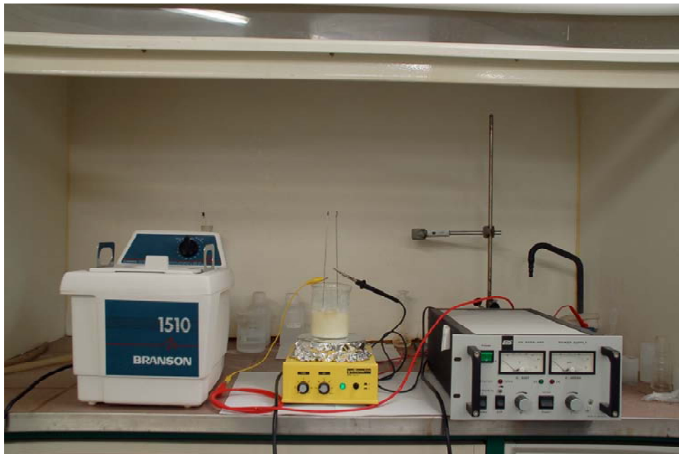
Figure 14: Representative image of the equipment used in this work for the EPD process. Left dispositive: ultrasonic bath; Middle dispositive: two electrodes cell, one positively charged and other negatively charged. Right dispositive: voltage supply. [Adapted from reference 40]
