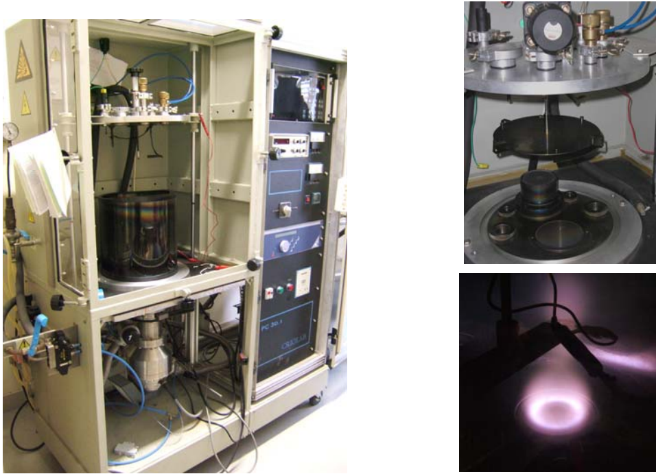
Fig. 3.6 – Different views of the experimental set-up for the D.C. magnetron sputtering deposition from Physical Department at Aveiro University.
