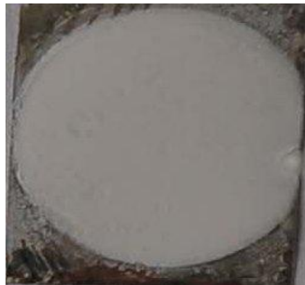
Figure 6-5: Surface morphology of BNT films deposited in acetone suspension media with triethanolamine, under 60V for 1min.
