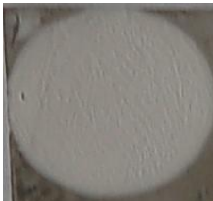
Figure 6-3: Surface morphology of BLT films deposited in ethanol suspension media with HNO 3 , under 100V for 1min
