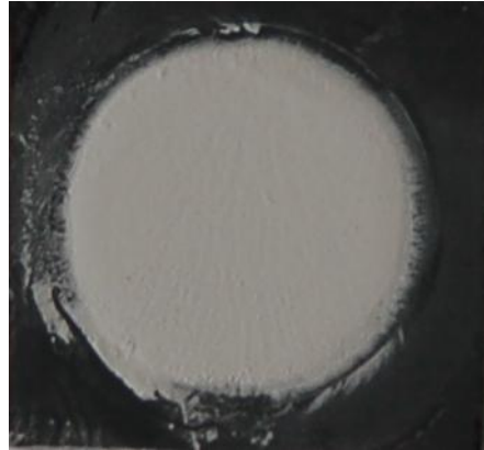
Figure 6-4: Surface morphology of BLT films deposited in acetone suspension media with triethanolamine, under 60V for 1 min.
