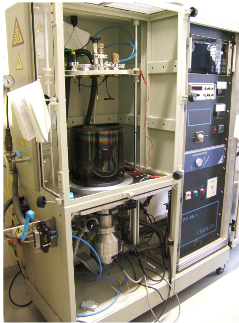
Figure 2: DC magnetron sputtering used in this work (Physics Dep., University of Aveiro).
