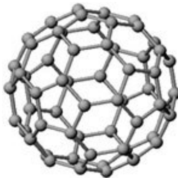
Figure 3: Schematic of a C 60 fullerene molecule [2]
