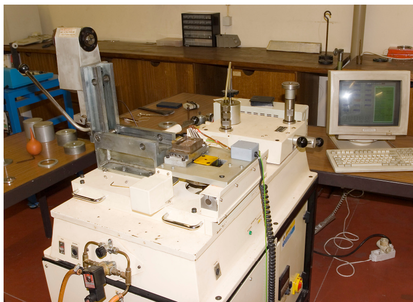
Figure 1: Tribometer with a ball-on-flat geometry (Mechanics Dep., University of Minho, Guimarães)
