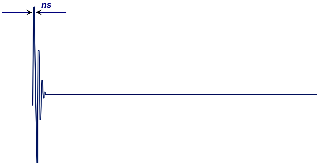
Fig. 23. Impulse response of a PA presenting short term memory effects, presented in [39].
