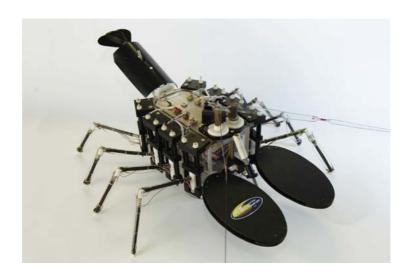
Figure 2.6: Example of an underwater biologically inspired robot, RoboLobster [12].
