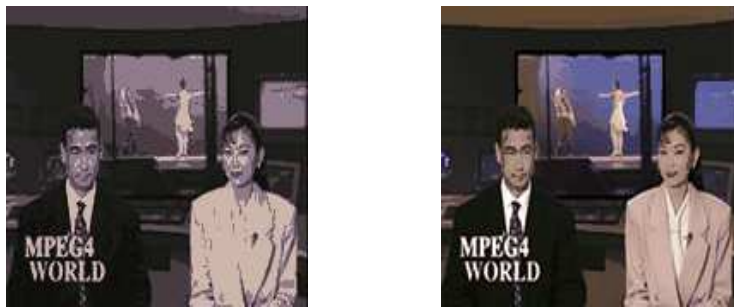
Figure 1.2: Two examples of color indexed images. Both images are the first frame from the video News, found at [3], where the first one has been reduced to a palette of 8 colors, whereas the second one has a colormap of 256.
