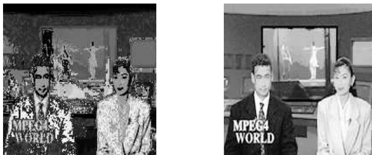
Figure 3.2: Two images of indexes of the same frame after color quantization. On the left, it is presented the image without palette reordering and on the right, the same image after the reordering process.
