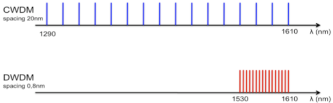
Figure 2-14 Representation of a 16 channels CWDM and DWDM systems
