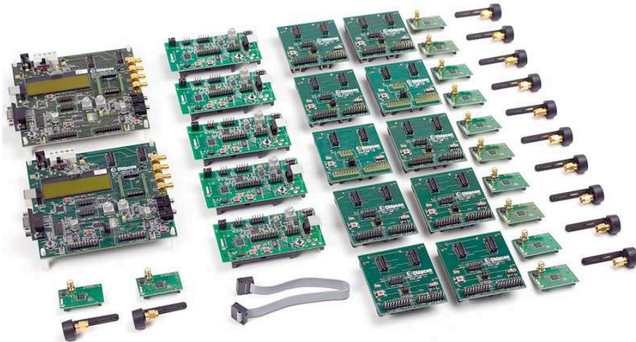
Figure 22: Chipcon Development Kit for Texas Instruments CC2430 content [CHI03]
