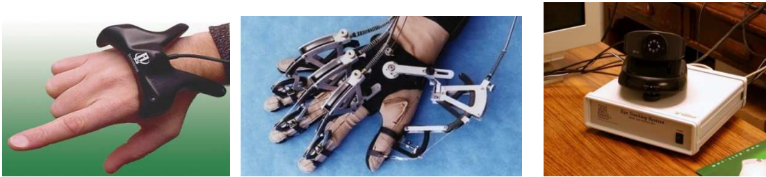
Figura 2 – a- Motion tracker [ Http://Www.Sti.Nasa.Gov/Tto/ , 2008]; b- Data glove [ Http://Www.Textura.Org/ , 2007]; c- Eye tracker [Live.Ece.Utexas.Edu, 2008].
