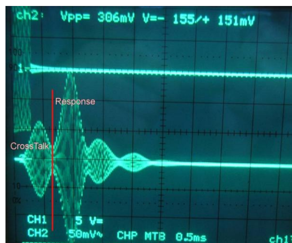
Figure 3-6: Direct path and response components (echo) of the received signal
