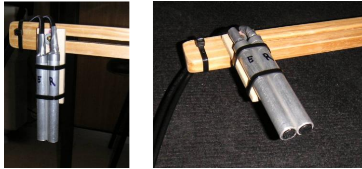
Figure 3-3: Emitter and receiver placed inside aluminum tubes
