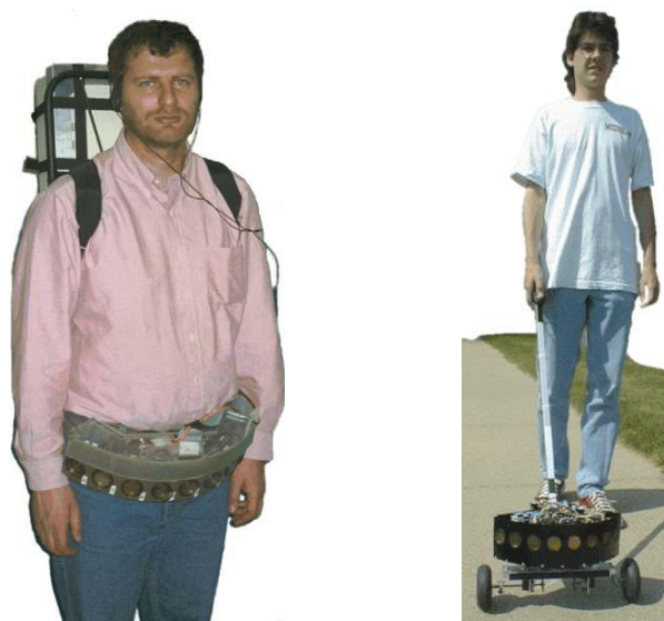
Figure 2-5: NavBelt and GuideCane
