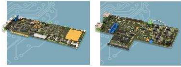
Figure 5.3: Sequans WiMAX development kit, from [Com07b]
