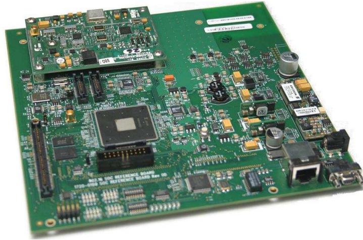
Figure 5.2: Fujitsu Fixed WiMAX development kit, from [Ame07]
