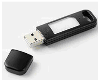
Figura 37: Axalto Reflex 530 E-gate Smart Card Enabler (Cyberflex e-gate 32k card chip)
