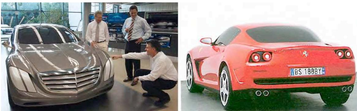
Figura 57 – Esquerda: Mercedes Benz, modelo integral em barro, à escala 1:1, do Mercedes Benz F700 Concept Car, <http://www.carbodydesign.com/archive/2007/09/26-mercedes-benz-f700-concept-design/>; direita: Ferrari, modelo à escala 1:4, em espelho, do Ferrari 599 GTB Fiorano, <http://autodesign.socialblog.us/2008/09/10/yesterday-series-ferrari-599-gtb-fiorano-the-design-story/#more-69>.
