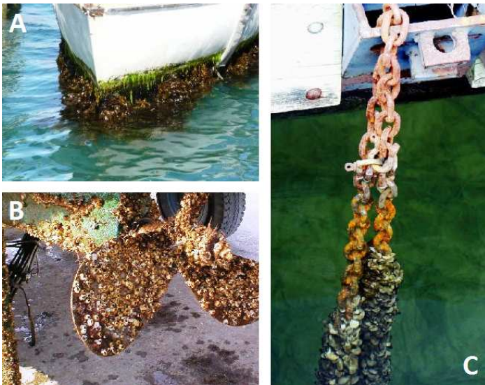
Figure 1.2 Pictures of marine biofouling on: (A) a ship hull, (B) a propeller of a vessel in dry dock and (C) the submerged portion of an anchor chain.
