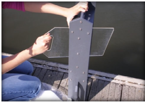
Figure 6: Performing Glass-Plate sampling, SML.
