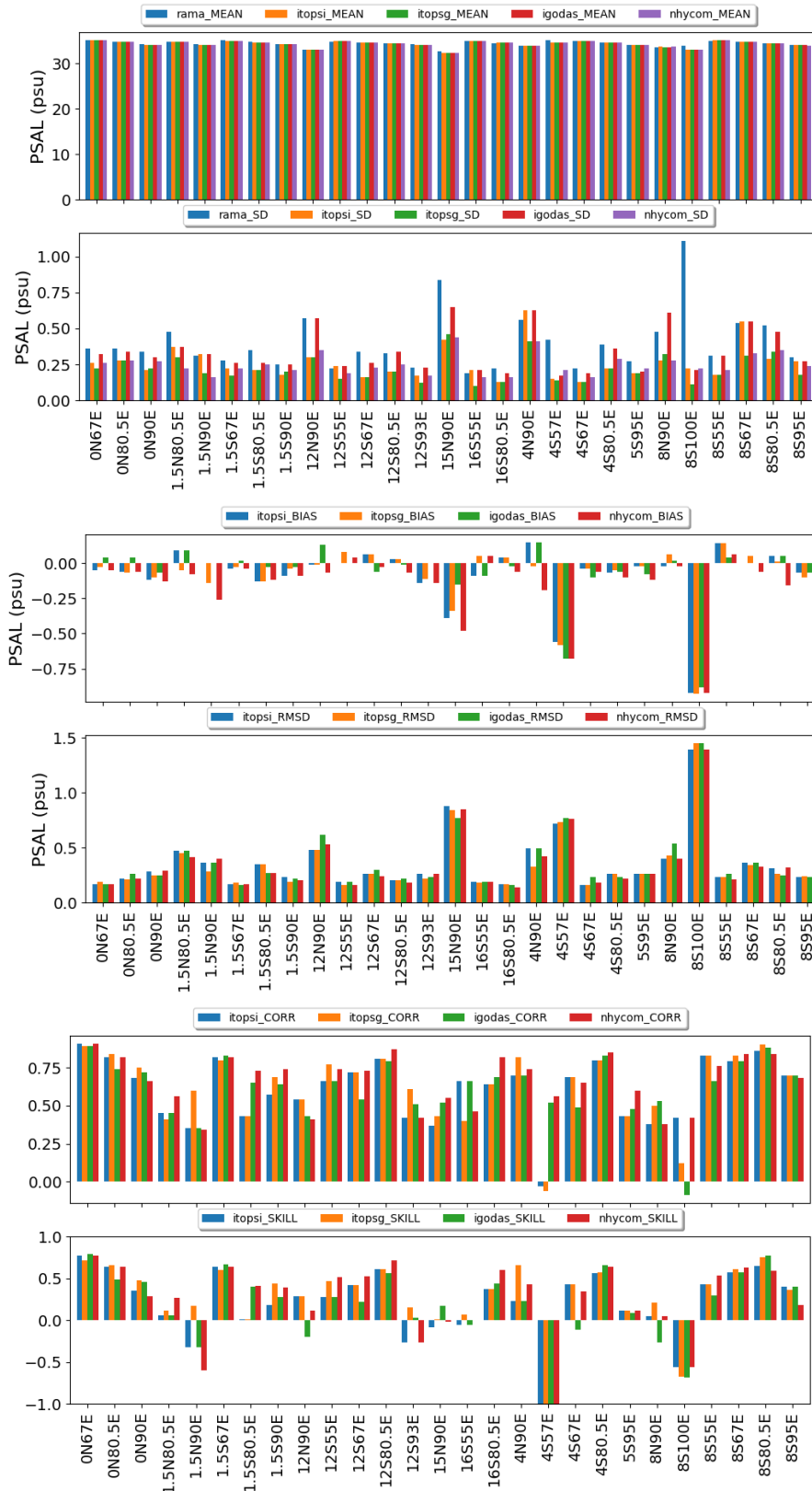
Figure 12: Comparison of SSS from 4 models in terms of mean, standard deviation, bias, rmsd, correlation and skill score with respect to RAMA buoys for the period 2012-2016.
