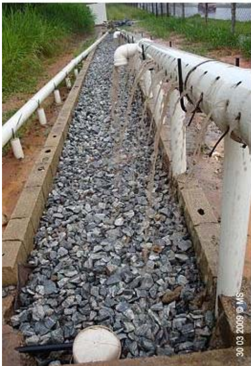
Figure 1. Configuration the experimental infiltration trench (Silva et al., 2010)
