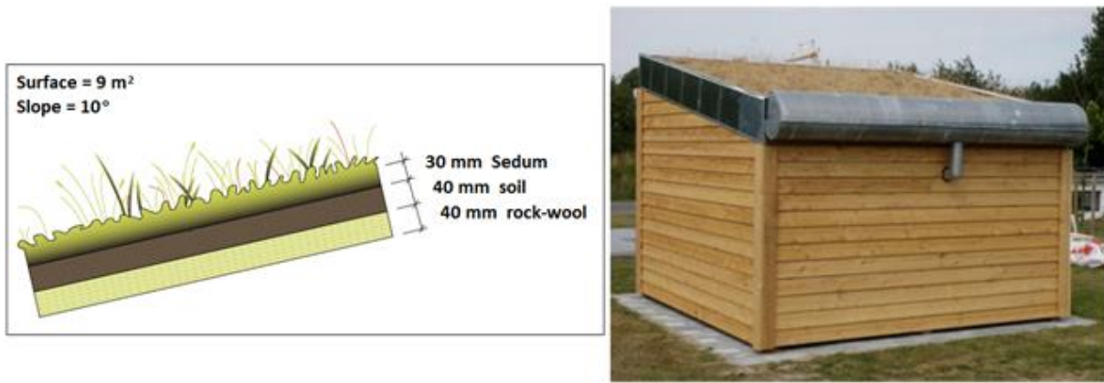
Figure 1: monitoring green roof. Cross section (left), the substrate is made of a mix of mineral soil. Overall test setup (right).
