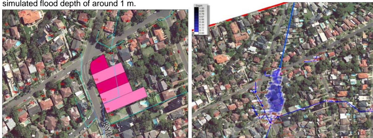
Figure 5 Recorded 1975 Flooding of properties (left) and Simulated 1975 Flood Event (right)
