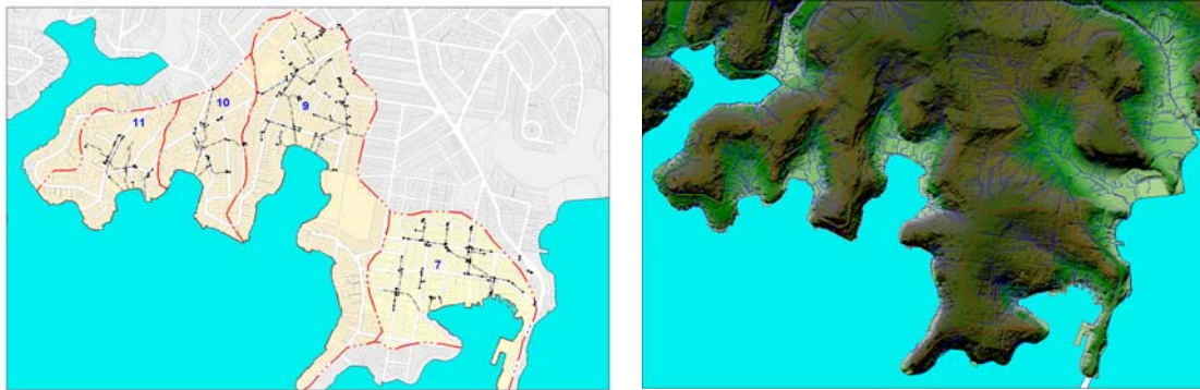
Figure 2 Drainage System (left) and Digital Elevation Map (right) showing naturalised streams
