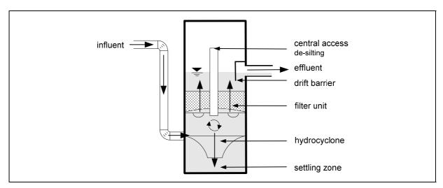
Figure 2: Schematic diagram of the 3P treatment facility
