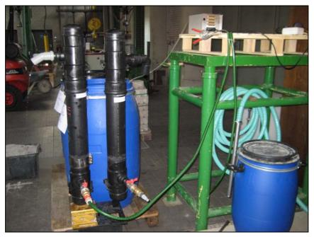
Figure 4: Photo of the heavy metal test in columns
