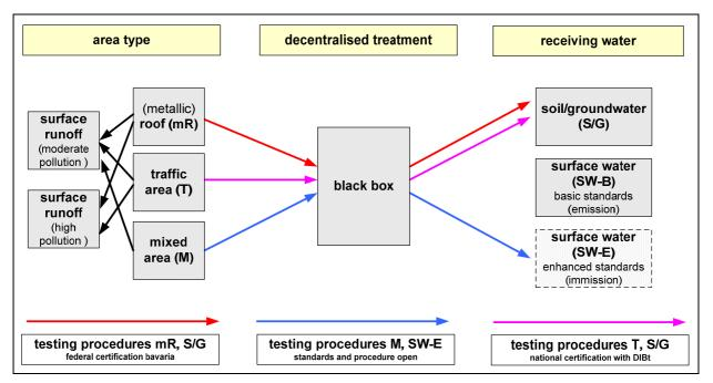
Figure 1: Illustration of typical applications for/use of decentralised treatment; mR: metallic roof; T: traffic area; M: mixed area; S/G: soil/groundwater, SW-B: surface water, basic standards, SW-E: surface water, enhanced standards, DIBt: Deutsches Institut für Bautechnik [adapted from DWA, 2010]
