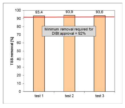
Figure 5: TSS-removal in three tests on the 3P-facility
