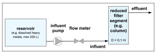
Figure 3: Schematic diagram of the heavy metal test in reduced-size filter segment (e.g. columns)
