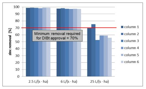
Figure 7: Removal of zinc in six filter columns and three test rain intensities
