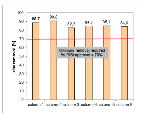
Figure 8: total removal of zinc in six filter columns
