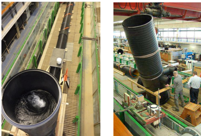
Figure 2: The SediPipe 600/24 operated in the lab at TU-Delft [1]
