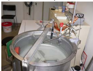
Figure 2 : Water tank and instrumentation.
