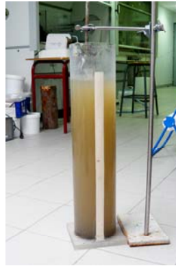
Figure 3 : Settling column filled with wastewater and the ultrasonic transducer on top.
