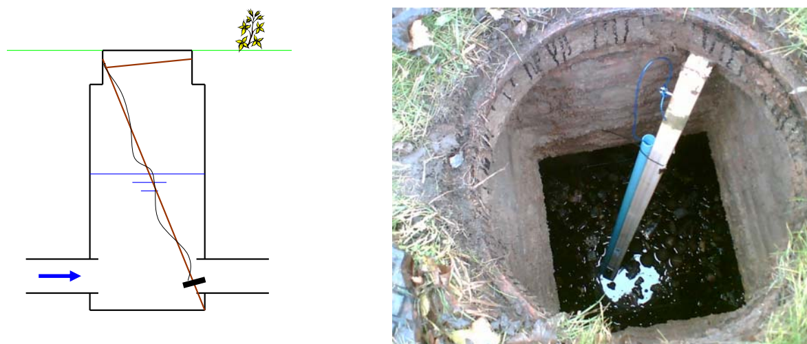
Figure 3. Left: Schematic of installation of sensor (water level, temperature and conductivity), right: picture of installed sensor in manhole (please note gross solids in manhole)
