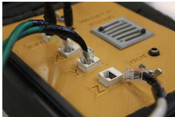
Figure 8. Sensors, Motors, Heaters and Fans all clipped into the Control box via Ethernet cables.
