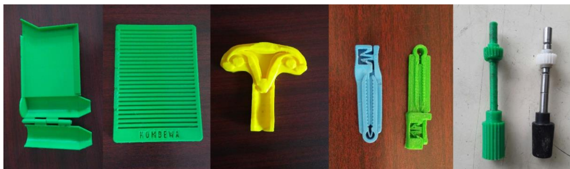
Figure 11. Examples of 3-D-printed medical parts created by the Kijenzi printer include, (from left to right), a pill sorter, a slide dryer, a uterine model, a replica of an umbilical cord clamps, and a replacement knob for a microscope.
