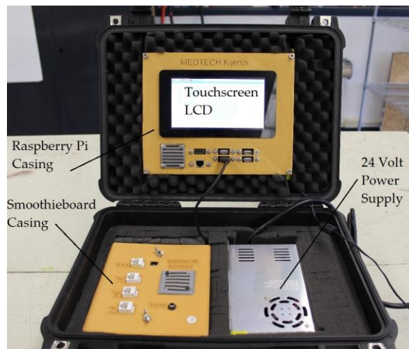
Figure 7. The Control Box for the Kijenzi 3-D printer with Liquid Crystal Display (LCD).
