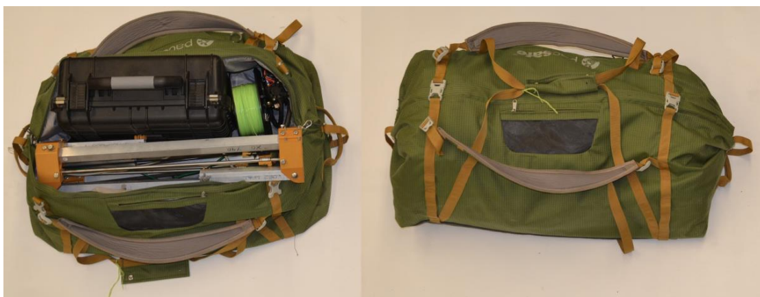
Figure 5. The Kijenzi 3-D printer can be disassembled and fit into a backpack or travel duffel.
