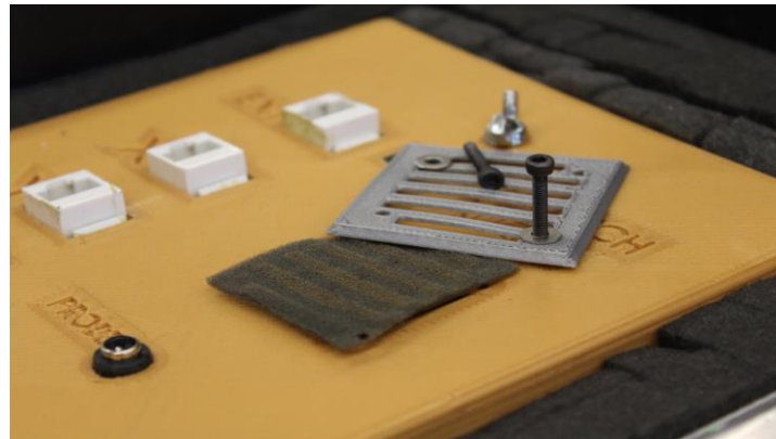
Figure 10. Fans with dust filters were effective at protecting electronics.
