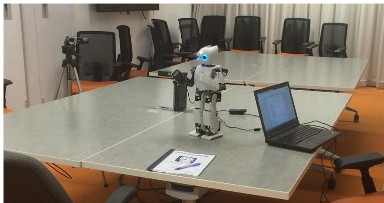
Figure 4. The experiment setup, consisting of a video camera (left), Kinect (behind robot), OP2, a laptop to operate OP2, and the informed consent packet.
