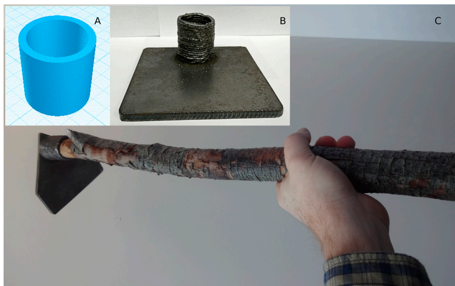
Figure 2. A hoe (A) 3-D model of handle hold; (B) metal 3-D printed part on substrate; and (C) finished hoe, cut and mounted to wooden handle.
