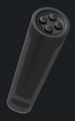
SENS utilizes an elastic strap on the back of the controller to keep it attatched to your hand while capacative zones track your fingers. With SENS, you can reach out and grab objects in the virtual world.
