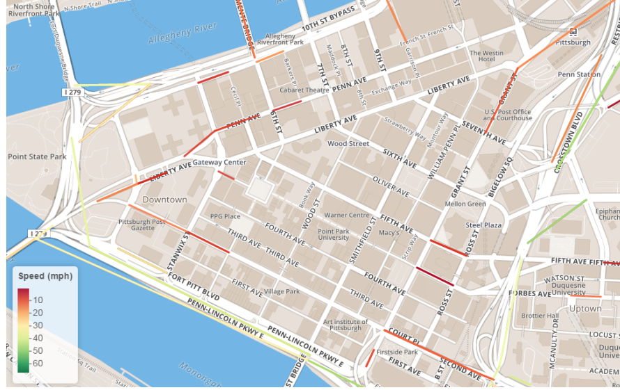
FIGURE 6.2: Speed distribution along road segments covered by my TMC dataset in downtown Pittsburgh on a typical weekday in August, 2014 at 8 a.m.
