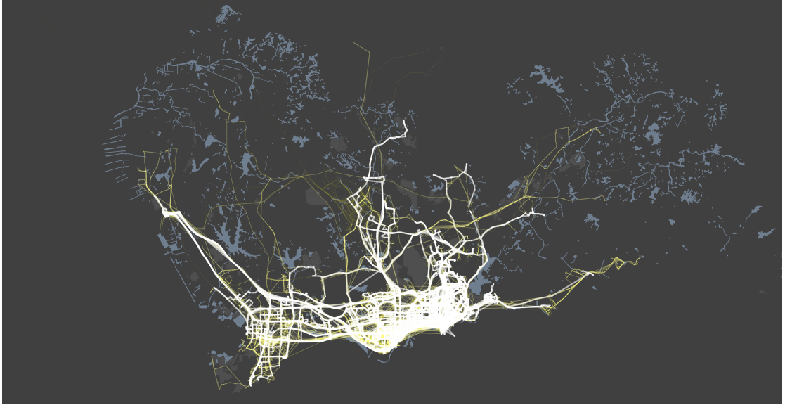
FIGURE 1.1: Visualization of almost 180,000 taxi trip trajectories in Shenzhen, China for the whole month of September, 2009. Each trajectory is a sequence of fine-grained GPS samples of locations and timestamps from the origin to the destination of the trip. Brighter areas correspond to higher and denser mobility demands in the road network.
