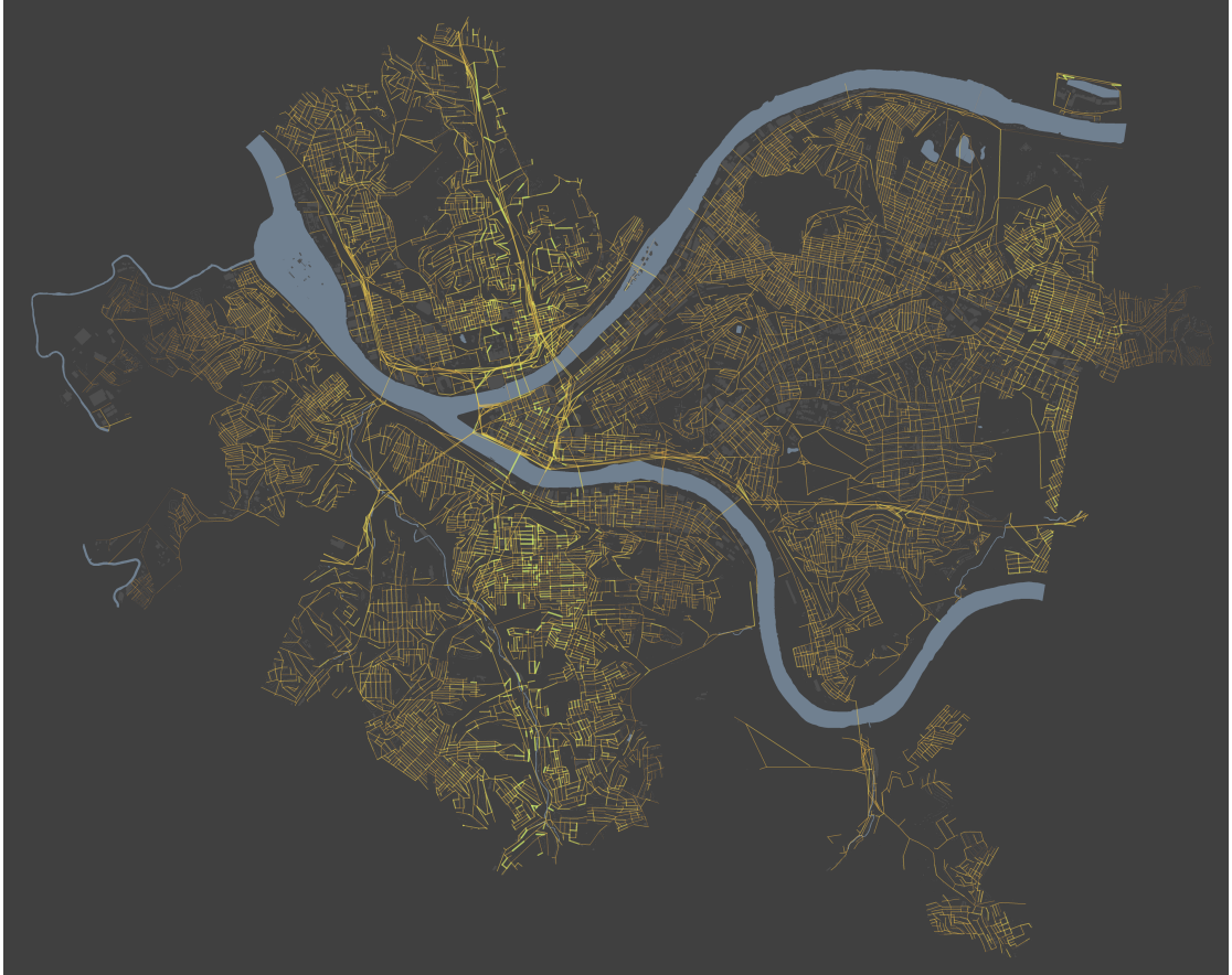
FIGURE 3.5: Visualization of the daily average traffic speed values along road segments in Pittsburgh, P.A. in August, 2014. Brighter colors illustrate higher speeds. Dark areas are either outside the city's boundaries or where no speed values were recorded.
