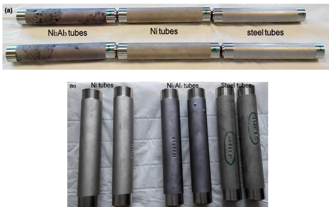
Figure 1. Appearance of the test tubes for (a) Esshete 1250 and (b) TP347H.
