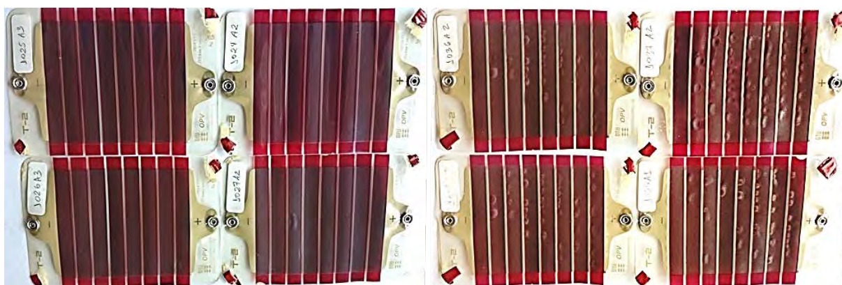
Figure 4.15 - AgNW-OPV-PT-PEDOT samples (left) and AgNW-OPV-PT-Ag (right) under ISOS-L-3. The four samples with PEDOT:PSS back electrode had no bubbles formed and the four samples with Ag-grid back electrode had extensive bubble formation. Adapted from [16].
