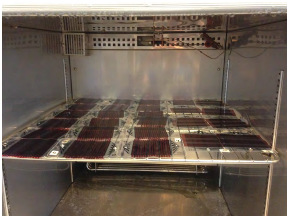
Figure 7. A photograph of the carbon-based freeOPV modules in the Thermotron chamber for ISOS-D-3 testing.
