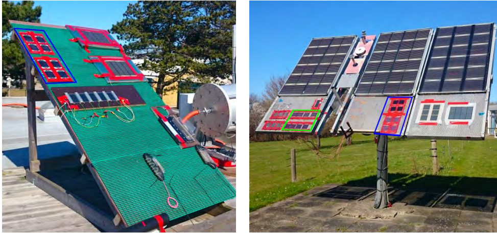
Figure 4.4 - Fixed (left) and tracked (right) platform for outdoor tests. Some of the samples used in this work are marked with blue (ISOS-O-1) and green (ISOS-O-2) squares.
