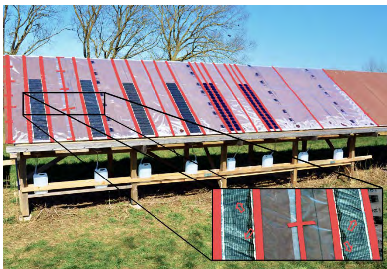
Figure 5.1 - Rain run-off experiment setup at DTU, Risø campus (Denmark), used to study the emission of elements to the environment from OPV during operation and failure. The inset shows the damage provoked in the first two Ag-OPV samples, simulating a worst case scenario. Reprinted with permission from [4].
