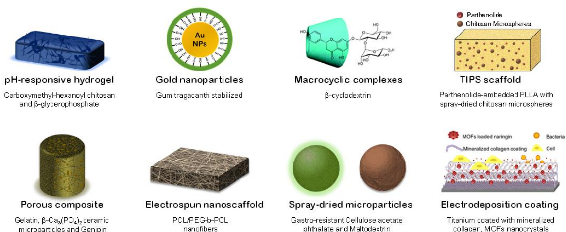
Figure 6. Overview of current strategies for Naringin incorporation into specialized biomaterial-based platforms. Representative images of literature reports are presented, except for the electrodeposition coating approach which was adapted from the respective reference 62 . TIPS – Thermal-induced phase separation. MOF – Metal-organic framework.
