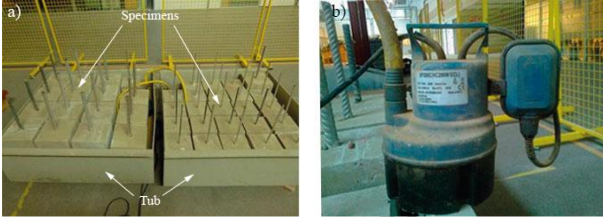
Fig. 2. a) PVC tubs filled with specimens. b) pumping equipment.
