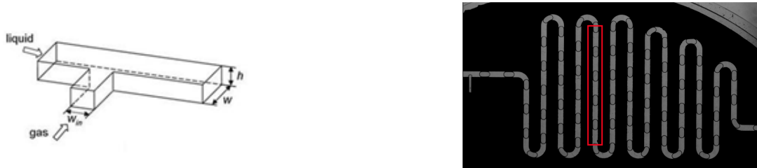
Figure 2: Contacting section: side entering T-junction, channel geometry: meandering microchannel with w_{l,in} = 1 \text{ mm} = w , w_{g,in} = 525 \mu\text{m} , h = 400 \mu\text{m} , d_h = 571 \mu\text{m} , l \sim 30 \text{ cm}
